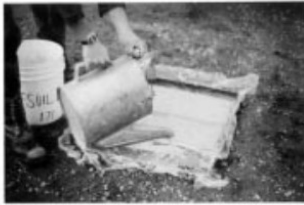
FIG. 4 Sand Being Poured Into the Template
